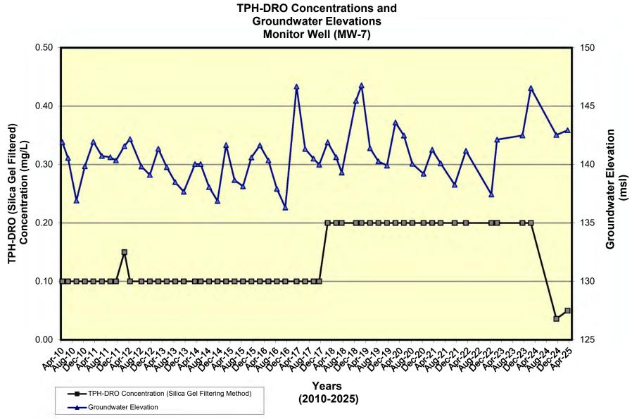
NOTE: TPH DRO Reporting Limit (0.1 mg/L April 2010 - Nov 2017; 0.2 mg/L Feb 2018 - Feb 2024; 0.036 mg/L in Nov 2024; and 0.050 in Mar 2025) If Dry, Well Bottom = 127.04 ft msl. Dec 29, 2020 and Mar 17, 2021 elevations are estimated. New reference elevation is needed.
