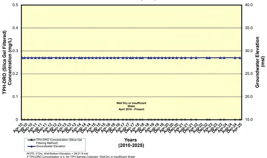
TPH-DRO Concentrations and Groundwater Elevations Monitor Well (MW-6)
