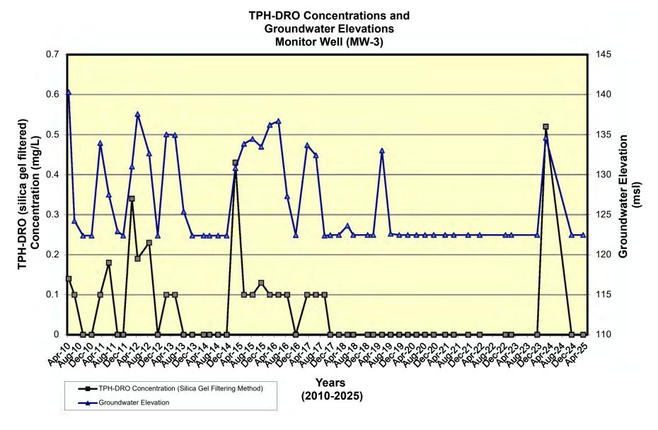
NOTE: If Dry, Well Bottom Elevation betwee 122.38 and 122.46 ft msl over time. If TPH-DRO Concentration is 0, No Sample Collected, Well Dry or Insufficient Water
