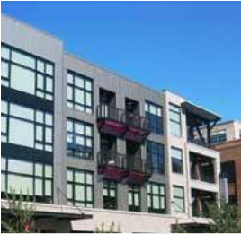
Example of photo illustrating a building façade with a distinct base and varying treatment to breakup building mass.
