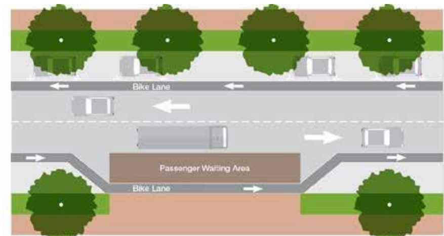
Figure 3.3 Floating Bus Stop and Bike Channel Design
