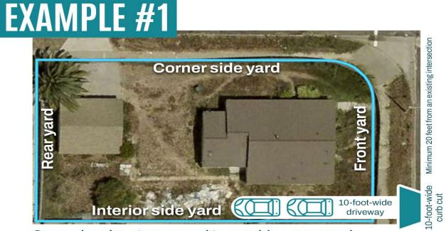
Second curb cut proposed to provide uncovered parking in the interior side yard setback.
