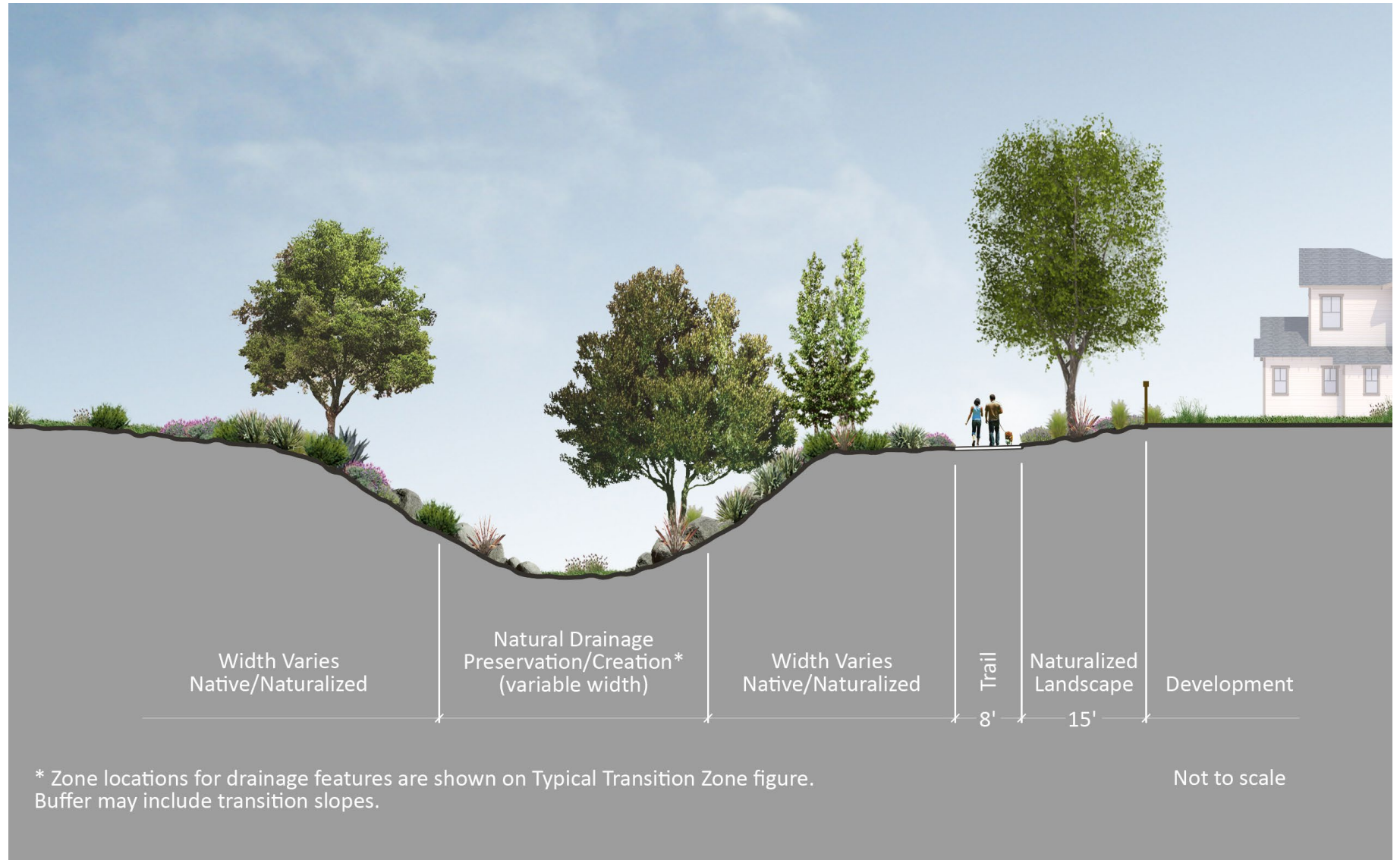
Figure 3-23 Typical Natural Drainage Zone w/ Greenway Trail
