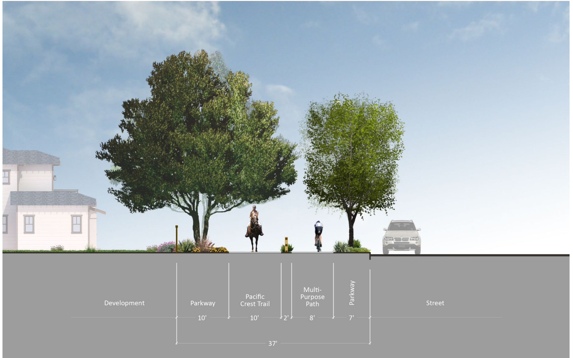
Figure 3-39 Typical Cross-Section of Pacific Crest Trail or a Regional Trail
