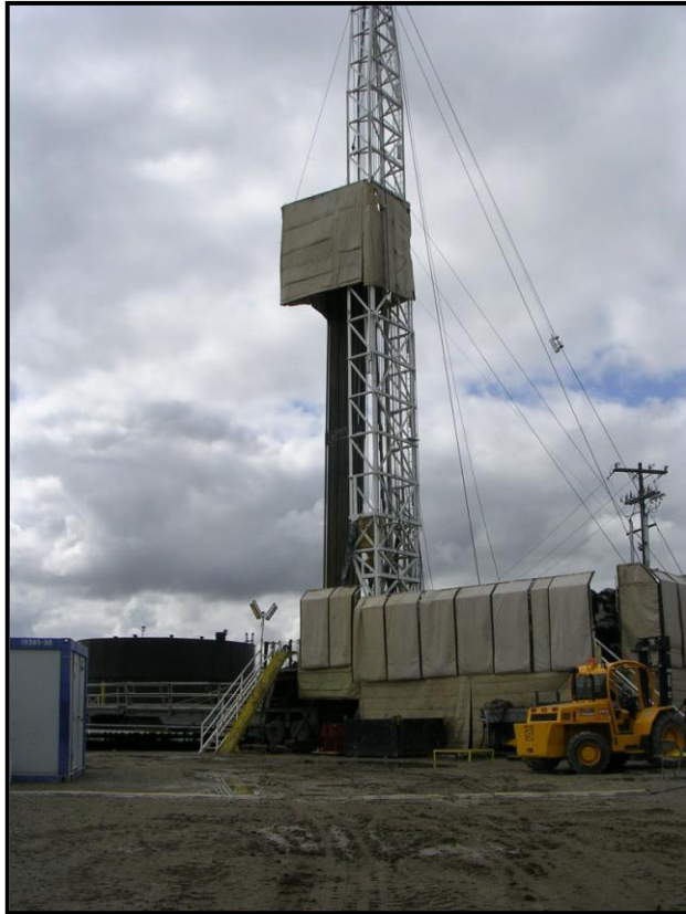
Drill rig with noise abatement pads
