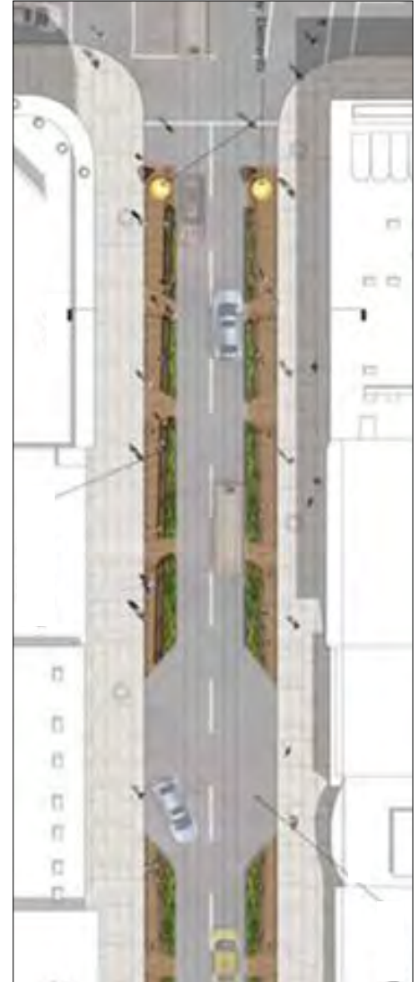
These conceptual parklets repurpose on-street parking to useable open space and landscaping without reducing the number of travel lanes (Conceptual layout by RHAA).
