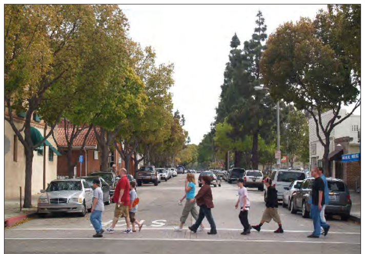
A crosswalk can be defined by striping and/or a change in paving material.
