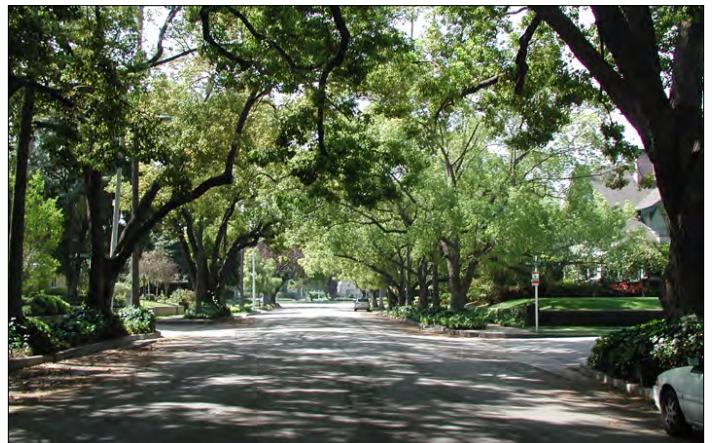
Street trees reduce the visual width of this 40-foot wide street and, along with the mottled pattern of dark and light that is cast on the roadway, encourage motorists to slow down.
