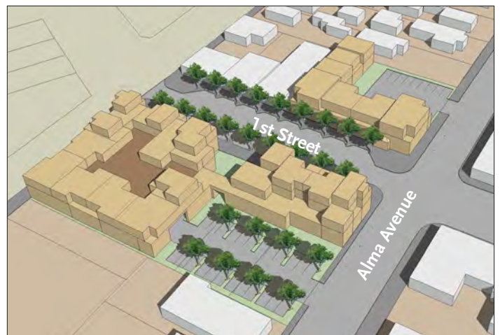
Conceptual massing of 1st Street with two- and three-stories of housing over retail and office uses, with parking placed in the back
