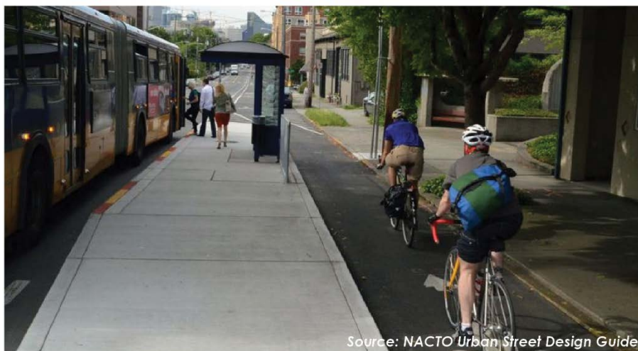
FIGURE 6.20: FLOATING BUS STOP AND BIKE CHANNEL IN
