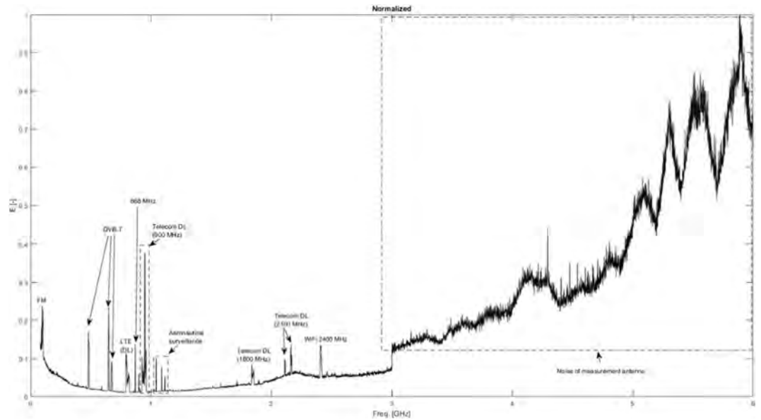
Figure 6. Overview measurement of electric field strength (normalized to maximally measured electric field strength), between 0.8 and 6 GHz, in Aalter. The wireless technologies associated with the different peaks are indicated in the figure as well.
